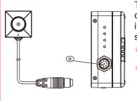
To connect the camera, plug the camera's connector end into (8) insert fully in to the socket and screw firmly in to place
